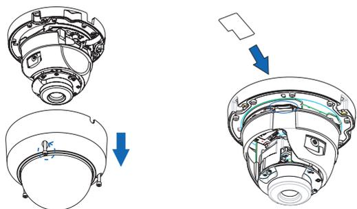
3. Install the mounting paper according to the monitored area.
