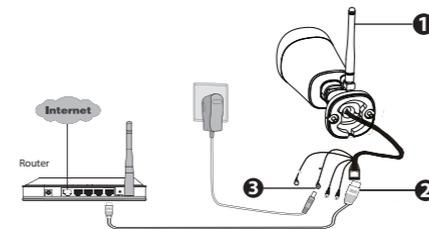
**Note:** We highly recommend that you first begin the setup process by connecting your camera to your Internet router with an Ethernet cable. After setup is successful, you'll be able to unplug the cable and login to your wireless network for WiFi operability.
