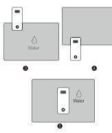
The above situations are the water leak or water presence event is triggered by the Sensor, when the water recedes from the Sensor, the water leak event will be cleared and then the Sensor will
